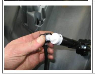
79. If headlamp washers are fitted, reconnect plumbing connections then attach the plumbing back to vehicle, routing rubber tubing along underside of vehicle grille crossmember, cable tie in position, taking care not to apply too much squeeze on tube with cable ties, as this will cut off flow.
