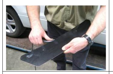
54. Apply rubber mould to edge of winch hole cover panel and trim off excess.
