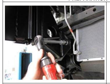
38. Fit impact absorbers to chassis ends using *fine thread M10 x 1.25P x 30 bolt* and washer sets supplied, note that the brackets are handed, slide them towards the centre of the vehicle on the adjustment slots *do not do up tight*
