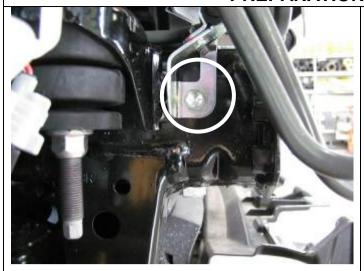
29. **PETROL MODELS ONLY:** Remove clamp from power steering pipes, by undoing the M10 bolt into the side of the chassis and the bolt holding the clamp plate. Set aside as this bracket will be reused
