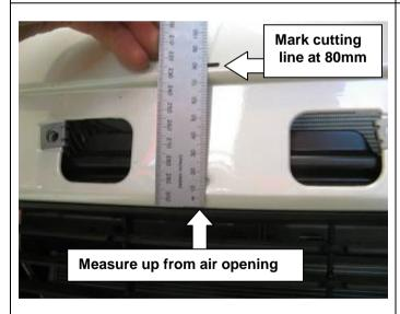
7. Mark a position for the centre of the cutting line at the centre front of the bumper above the lower opening in bumper at 80mm as shown.
