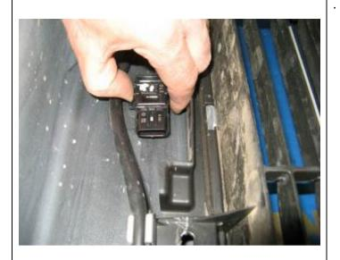
22. If parking sensors fitted, mark each sensor for identifying position in bumper, then carefully remove sensors, disconnecting from the harness first, then unclipping the sensor from the holding sleeve, finally remove the sleeves from the bumper holes
