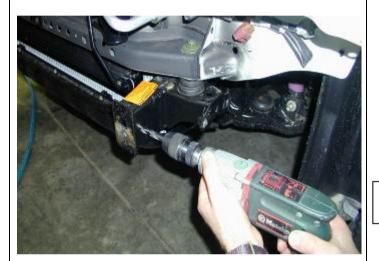
30. Using a power drill with Dia13mm bit, drill out captive nut in hole immediately behind chassis flange as shown, for both RH and LH chassis ends
