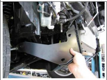
34. Fit handed specific side braces as shown, locating over the captive nuts at the rear of the chassis.
