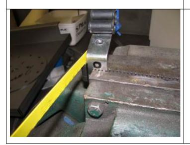
42. **PETROL MODELS ONLY:** Modify the clamp plate by cutting off the flange as shown then drilling a Dia 8.5 hole 8mm from the bend as shown
