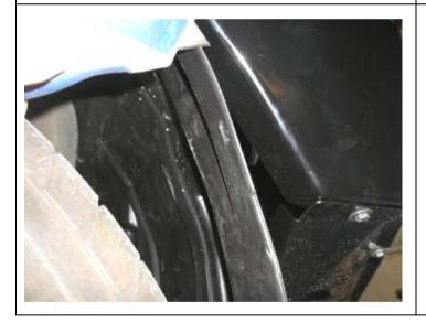
92. Trim the outer edge of the fender liner as shown so that it will clip in behind the wing
