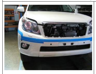
11. Note that the cutting line is co incident with the lower edge of the 50mm tape, *this is critical.*
