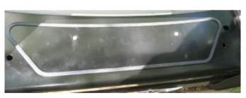
55. Fit panel to top face on bull bar using stainless steel 2 x M6 dome head screws and stainless steel flat washers and flange nuts.
