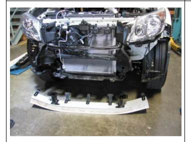
27. Remove reinforcing beam at mounts to chassis by undoing the M10 fine thread bolts. Set beam aside, it will not be reused
