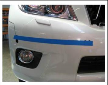
9. Apply some 25mm masking tape joining the cutting line positions from the most inboard position of the profile from the template to the mark on the outside of the 80mm marks across the centre of the bumper. Mark this line joining the two profiles, repeat for the other side of the bumper.
