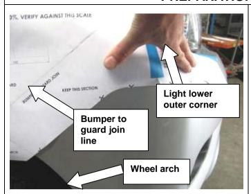
4. Carefully and accurately fit the template to the RHS of the bumper using the identified reference points aligning with the wheel arch, join of bumper and guard the head lamp outer lower corner and tape in position. Make sure the template sits as flat as possible on the bumper as any misalignment could affect the final cut profile accuracy on the vehicle.
