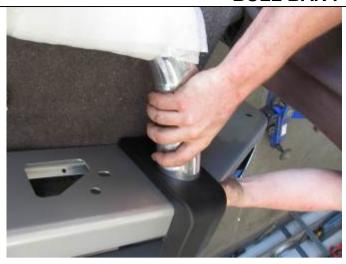
53. If fitting frame **P# 5121010**, locate frame as shown and then from below inside wings, secure with M12 x 50 bolts and washer sets
