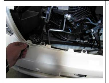
16. Remove the plastic rivets securing the top of the bumper
