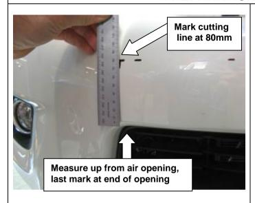
8. Continue to mark the cutting line position across the center of the bumper above the number plate location as shown out to the extent of the air opening in the bumper as shown. Continue to mark at 80mm as shown.
