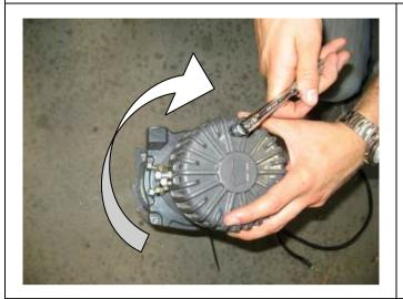
56. Rotate the winch motor 90 degrees as shown
