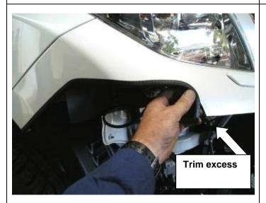
46. Fit pinch weld to cut area as shown, trim to length.
