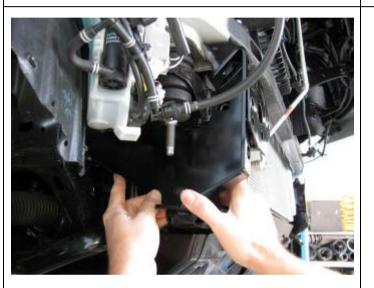
35. When side braces are fitted in position as shown, insert <u>fine thread M12 x1.25P x 30</u> <u>bolt</u> and washer sets into lowest hole position to chassis. There is an existing captive nut in chassis, **but do not do up tight.**
