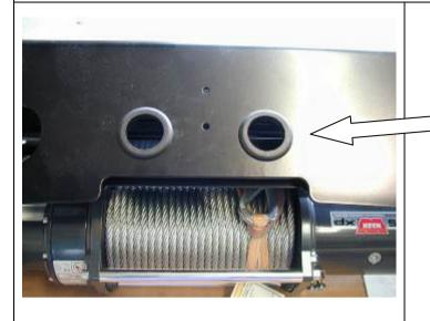
62. Insert the two rubber grommets into the top face of bull bar.
